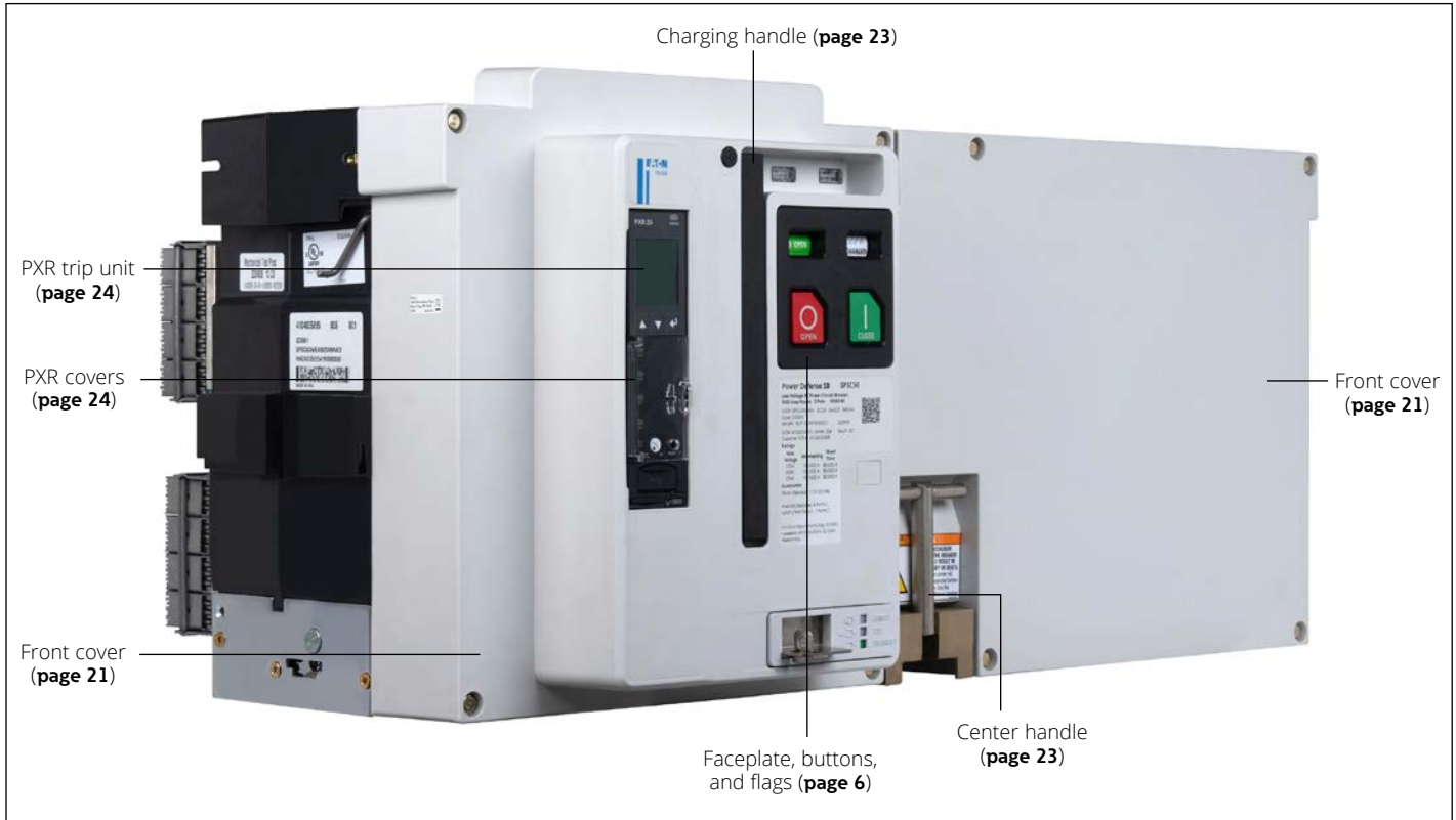
Figure 3. Magnum drawout breaker (ANSI 4000–6000 A, IEC 4000–6300 A), standard double wide; double narrow frame (4000–5000 A) available, not shown
