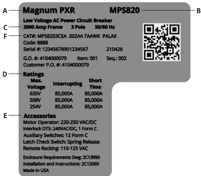
Magnum PXR nameplate (typical for Power Defense™ SB)
