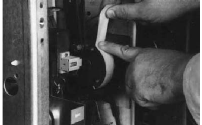
Figure 6-7 Wrapping Tape Up Around Cam
